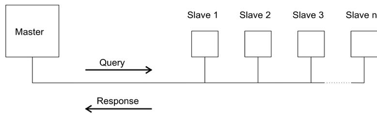
In the MODBUS Protocol the master can address individual slaves, or, using a special “Broadcast” address, can initiate a broadcast message to all slaves. The Integra Digital meter do not support the broadcast address.
