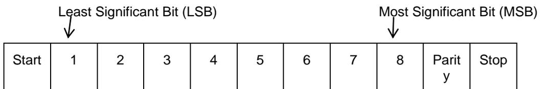
Transmit Character = Start Bit + Data Byte + 2 Stop Bits (11 bits total):
