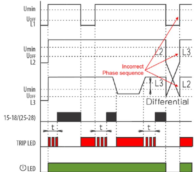
The time delay and differential trip levels help to prevent relay chatter as the monitored parameter fluctuates.
