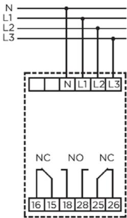
NC = Normally closed. Contact closed when relay de-energised.
