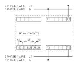
NC = Normally closed. Contact closed when relay de-energised.
