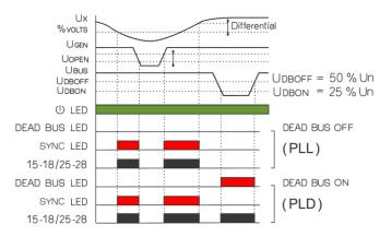
Ux = | UGEN - UBUS | ( VOLTAGE, FREQUENCY + PHASE ANGLE )
