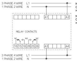
NC = Normally closed. Contact closed when relay de-energised.
