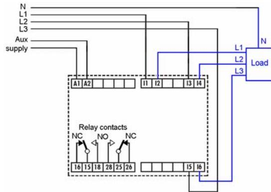
NC = Normally closed. Contact closed when relay de-energised.
