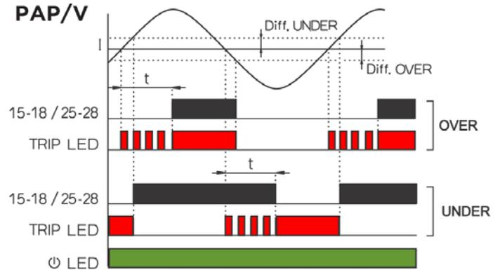
The time delay and differential trip levels help to prevent relay chatter as the monitored current level varies. As the relays have changeover contacts, the relay outputs can be inverted by wiring to the alternative terminals 15-16 or 25-26.
