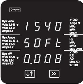
The second screen indicates the firmware installed in the display unit. This example states that the version is 0.008. The version on a particular unit will differ in line with ongoing development and improvements.
