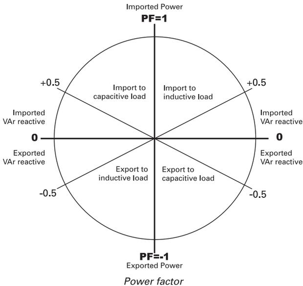
The polarity of the power factor reading indicates the direction of power flow:
