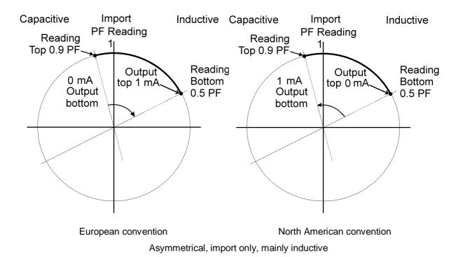
In the example above, the unit has an analogue output range of 0 to 1 mA, all power is imported and the load is inductive. The 1 mA Output range covers a reading power factor range of 0.6, from 0.9 capacitive to 0.5 inductive. The Output to Reading correlation is as follows:
