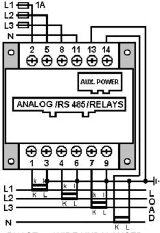
3-PHASE - 4 WIRE UNBALANCED LOAD with metered neutral L1 🕶 1A L2 🐢 L3 🗣 Ν 5 8 11 13 14 2 o 0 ⊕⊕⊕⊕⊕⊕ AUX. POWER -ANALOG /RS 485/RELAYS u . .  $\begin{array}{c} \bigoplus \bigoplus \bigoplus \bigoplus \bigoplus \bigoplus \\ 4 & 6 & 7 & 9 \end{array}$ ⊕ Ð O o з 1 L1 L2 ō P1 L3 Ã P1 N
