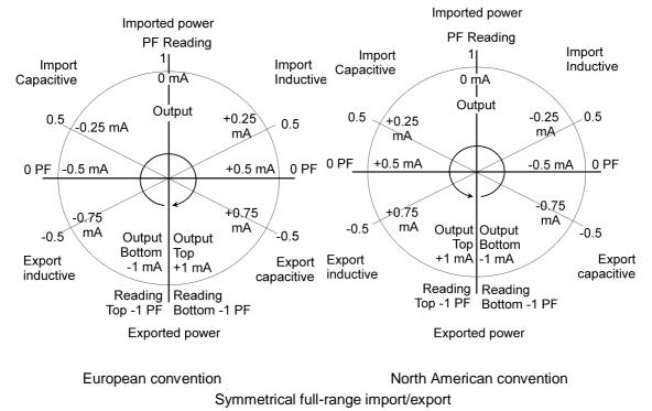
In this example, the unit represents the full range of inductive and capacitive loads on imported and exported power. The unit has an analogue output range of -1 to +1 mA. Both Reading Top and Reading Bottom are set to -1 power factor.
