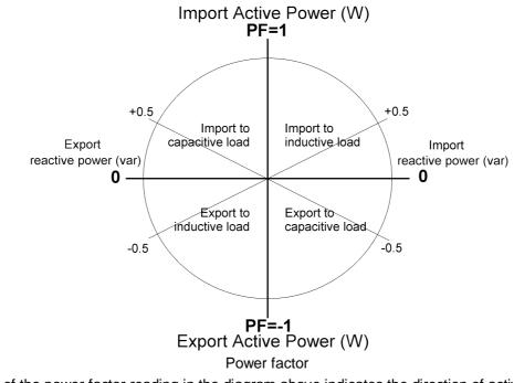
The polarity of the power factor reading in the diagram above indicates the direction of active power flow:
