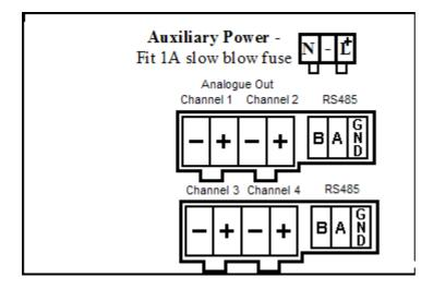
Note that the return(-ve) terminal for analogue outputs is common amongst all analogue channels. The analogue return is galvanically isolated from the RS485 ground.
