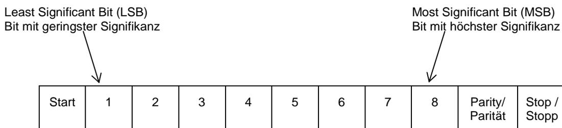
Transmit Character = Start Bit + Data Byte + 2 Stop Bits (11 bit total):
