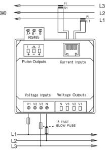
Please note for 3P3W configuration L2 is connected through the neutral and not V2.
