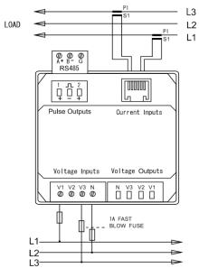
Please note for 3P3W configuration L2 is connected through the neutral and not V2.
