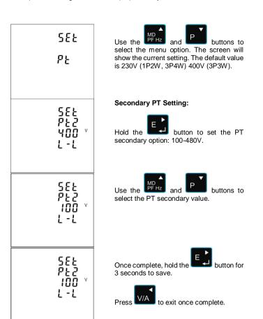
Note: The unit is able to measure from 57.7V AC L-N however PT2 must be set from 100-276V AC L-N.
