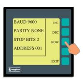
This screen allows the user to configure the parameters for the RS485 port. NOTE: Communicatios settings for Johnsons Controls are fixed and pre set. A pointer is shown next to the value being changed. The "INC" and "DEC" keys are used to increment and decrement the displayed value. The "ROW" key is user to move the pointer to the next parameter.
