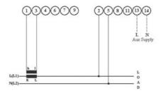
**Wiring** - Input connections are made directly to shrouded screw clamp terminal. Numbering is clearly marked on the plastic moulding. Choice of cable should meet local regulations. Terminals for both current and voltage inputs will accept up to 3mm2 x 2 diameter cables.
