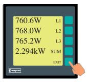
This will expand the active screen to full size. This screen remains until deactivated by pressing "EXIT" where it will return to the reduced active screen.
