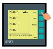
This screen assigns a parameter to each of the four screen lines.
