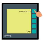
Press "UPDATE RATE". This screen allows the screen update time to be modified. The standard update time is approximately 100ms but users can progamme the Integra 2000 to override up to 20 updates thereby avoiding digi roll. Analogue and digital outputs are not affected by this feature. The bar flashes at the selected rate to assist selection.
