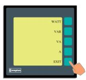
Press "WATT" to zero accumulated W.h. "RESET" will appear to the left indicating this choice has been made. A similar function is performed by the "VAR", "VA" and "A" keys.
