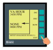
If any output is assigned to be "NONE", no pulses will be transmitted.
