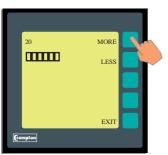
Press and hold the "MORE" or "LESS" buttons, this will increment the number on the far left or the screen.
