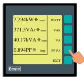
All the screen stages for "WATT" are repeated for "VAR" and "VA".
