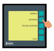
The "DIVISOR" screen enables a divide ratio of 10, 100 or 1000. This allows the user to program the unit to output a lower number of pulses according to the system requirements. For example, setting the divisor to 1000 will output kilowatt hour pulses, and setting the divisor to 1 will output Watt hour pulses.
