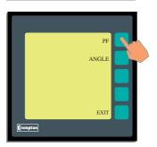
On pressing "**PF PA**" the display offers two choices for displaying the phase relationships: Power Factor ("**PF**") and Phase Angle ("**ANGLE**").
