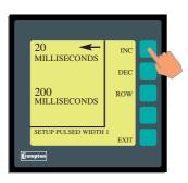
"INC" increases the value in 20mS increments up to a maximum of 200mS
