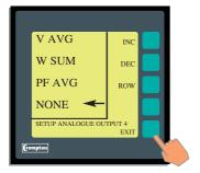
If any output is assigned to be "NONE", a zero value will be transmitted.
