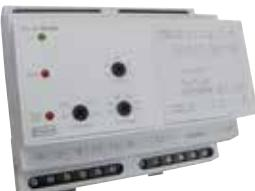
The synchro-check (paralleling) protector trip relay compares the voltage, frequency and phase angle of two supplies and operates a relay according to the state of synchronisation of the supplies. If the two supplies are not synchronised, the relay operates to provide a control output.
