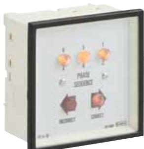
Electronic phase sequence indicators ensure correct phase rotation and the presence of all 3-phase supplies. Incorrect or loss of phase can cause serious damage in a wide range of electrical machines. Ship-to-shore supplies, mobile generators and remote installations are particularly vulnerable to this problem.
