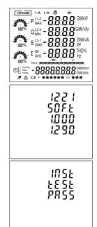
The first screen lights up all display segments and can be used as a display check.
