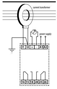
Residual current devices are used to detect dangerous ground fault currents before damage is caused to expensive power assets. The ELRP/S monitors the earth leakage current and compares it with the user selectable trip level. Should this level be exceeded, the relay will trip and with a response time of under 40ms, the supply can be disconnected before serious damage can occur.
