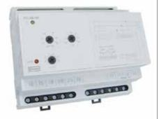
The Reverse Power protector trip relay monitors a single- or three-phase supply for reverse power and trips a relay if it detects reverse power ( $I \times \cos \Phi$ ) over a set limit. The relay output is typically used to prevent 'motoring' of a generator (where the generator turns the engine), which can damage the engine.
