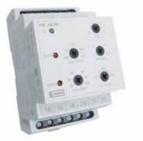
When the measured voltages moves outside the set point limit for longer than the time delay, the relay will operate giving an alarm control or tripping signal. The Protector can be used for under and over voltage detection, start standby generators, operation of mains failure units and switching standby suppliers. An illuminated red LED indicates a fault condition. The three-phase, three or four-wire models with protect each phase independently.
