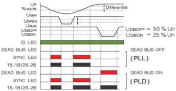
Ux = UGEN - UBUS ( VOLTAGE, FREQUENCY + PHASE ANGLE )
