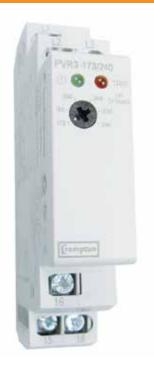
The phase sequence and phase failure protector trip relay is designed to monitor the correct phase rotation or sequence of a three-phase supply system. It provides protection against incorrect phase sequence, loss of one phase and under voltage. Two versions are available to suit either three-phase three-wire (PVR3) or threephase four-wire (PVR4) systems.
