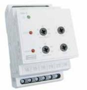
AC current protectors provide a continuous surveillance of monitored circuits and offer user adjustable trip points (set points) with time delay settings. When the current moves outside the set point limit for longer than the time delay, the relay will operate providing an alarm control or tripping signal.
