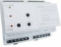
The synchro-check (paralleling) protector trip relay compares the voltage, frequency and phase angle of two supplies and operates a relay according to the state of synchronisation of the supplies. If the two supplies are not synchronised, the relay operates to provide a control output. The relay output can be used for alarm or control purposes.
