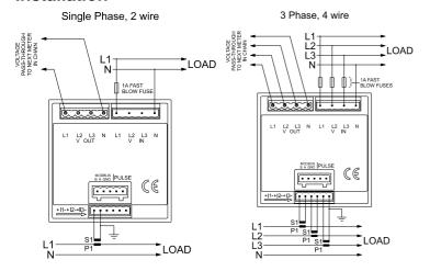
The unit may be mounted in a panel of any thickness up to a maximum of 6mm (0·25in). Leave enough space behind the instrument to allow for bends in the connection cables. As the front of panel enclosure conforms to IP52, it is protected from dripping water. The unit is intended for use in a reasonably stable ambient temperature within the range -10 to +55°C. Do not mount the unit where there is excessive vibration or in excessive direct sunlight.
