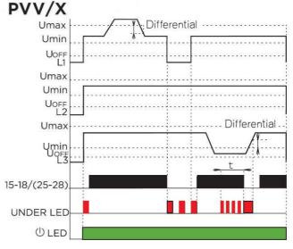
The time delay and differential trip levels help to prevent relay chatter as the monitored voltage level varies. As the relays have changeover contacts, the relay outputs can be inverted by wiring to the alternative terminals 15-16 or 25-26.
