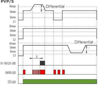
The time delay and differential trip levels help to prevent relay chatter as the monitored voltage level varies. As the relays have changeover contacts, the relay outputs can be
