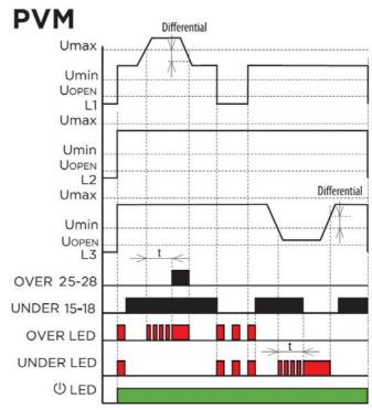
The time delay and differential trip levels help to prevent relay chatter as the monitored voltage level varies.
