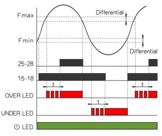
The time delay and differential trip levels help to prevent relay chatter as the monitored frequency varies.
