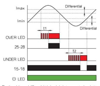
The time delay and differential trip levels help to prevent relay chatter as the monitored current level varies. As the relays have changeover contacts, the relay outputs can be inverted by wiring to the alternative terminals 15-16 or 25-26.
