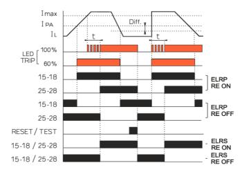
The time delay and differential trip levels help to prevent relay chatter as the monitored voltage level varies.
