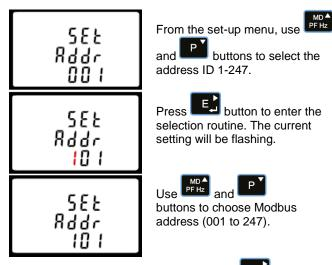
On completion of the entry procedure, press button to confirm the setting and press button to return the main set-
