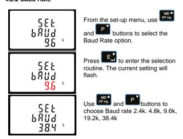
On completion of the entry procedure, press to confirm the setting and press to return to the main set up menu.
