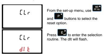
Press to confirm the setting and press to return to the main set up menu.
