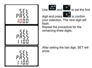
Press to exit the number setting routine and return to the Set-up menu. SET will be removed.
