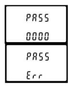
Setting up is password protected so you must enter the correct password (default '1000') before processing.
