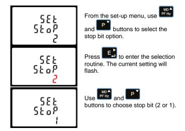
On completion of the entry procedure, press to confirm the setting and press to return to the main set up menu.
