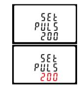
From the set-up menu, use and buttons to select the Pulse width option.
