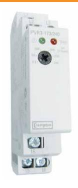
The phase sequence and phase failure protector trip relay is designed to monitor the correct phase rotation or sequence of a three-phase supply system. It provides protection against incorrect phase sequence, loss of one phase and under voltage. Two versions are available to suit either three-phase three-wire (PVR3) or three-phase four-wire (PVR4) systems.
