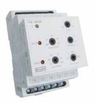
When the measured voltages moves outside the set point limit for longer than the time delay, the relay will operate giving an alarm control or tripping signal. The Protector can be used for under and over voltage detection, start standby generators, operation of mains failure units and switching standby suppliers. An illuminated red LED indicates a fault condition. The three-phase, three or four-wire models with protect each phase independently.
