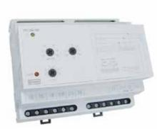
The Reverse Power protector trip relay monitors a single- or three-phase supply for reverse power and trips a relay if it detects reverse power (I x cos  $\Phi$ ) over a set limit. The relay output is typically used to prevent 'motoring' of a generator (where the generator turns the engine), which can damage the engine.
