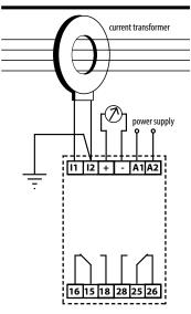
Residual current devices are used to detect dangerous ground fault currents before damage is caused to expensive power assets. The ELRP/S monitors the earth leakage current and compares it with the user selectable trip level. Should this level be exceeded, the relay will trip and with a response time of under 40ms, the supply can be disconnected before serious damage can occur.
