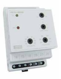
The phase balance, sequence and voltage protector trip relay, is designed to monitor a three-phase supply for phase imbalance, low or missing phases or incorrect phase sequence and to trip a relay if it detects any anomaly. Two versions are available to suit either three-phase three-wire (PSF/G3) or three-phase four-wire (PSF/G4) systems.
