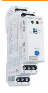
The Thermistor protector trip relay monitors the temperature of a motor using the PTC sensor (positive temperature coefficient resistor) or thermostat (TK) switch built in to the motor winding. Relay contacts can be used to disconnect the supply to the motor should it overheat. LEDs indicate mains on and fault status.
