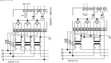
A fuse of 6A is recommended for the line protection. Current transformers must not be operated with open terminals since dangerous high voltages might occur which may result in personal injuries and property damage. In addition to this, the transformers are exposed to thermal overload.
