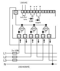
A fuse of 125A is recommended for the line protection. Wire N needs to be connected to the meter.
