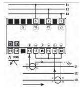
DRK-3PCT Three-phase CT connected 5A(\*) four-wire system
