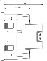
The Integra Ci1 energy meter is specially designed and developed as a cost affected watt hour and VAr hour meter to complement the current Crompton Instruments Ci meter series. The Integra Ci1 self-contained 96mm DIN panel mounted Watt hour, VAr hour meter measures the real consumption of active and reactive energy to Class 1.0 accuracy.
