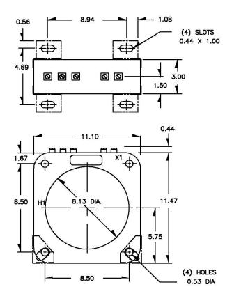
20 turns 600:5A 50 40 10 (X4 (X3) (X2) 1200:5A 80 100 20 40 turns (X2 (X4) 2000:5A 100 80 turns 60 160 (X2) (X5) (X4) (X3) 3000:5A 100 60 240 200 turns (X4) (X2 (X5 (X3 4000:5A 200 200 300 100 turns (X4) (X2) (X5) (X3 5000:5A 200 400 100 300 turns (\$5) (\*4) (X3) (2) (X1) MARKED RATIO (MR)
