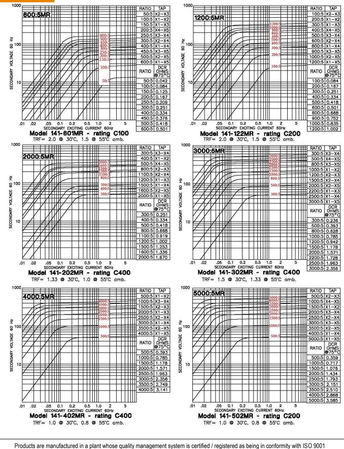
APPLICATION: Metering FREQUENCY: 50-400 Hz. INSULATION LEVEL: 600 Volts. 10 kV BIL. full wave WINDOW DIAMETER: 6.31" APPROXIMATE WEIGHT: 3 lbs.
