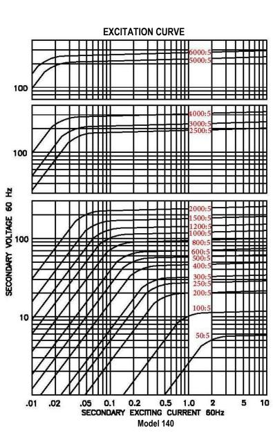
APPLICATION: Relaying and metering FREQUENCY: 50-400 Hz. INSULATION LEVEL: 600 Volts. 10 kV BIL. full wave WINDOW DIAMETER: 8.13" APPROXIMATE WEIGHT: 22 lbs.
