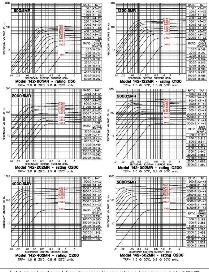
APPLICATION: Relaying and metering. FREQUENCY: 50-400 Hz. INSULATION LEVEL: 600 Volts. 10 kV BIL. full wave WINDOW DIAMETER: 7.31" APPROXIMATE WEIGHT: 60 lbs.
