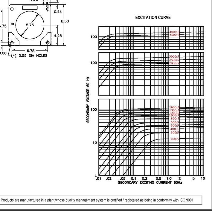
APPLICATION: Relaying and metering. FREQUENCY: 50-400 Hz. INSULATION LEVEL: 600 Volts. 10 kV BIL. full wave WINDOW DIAMETER: 5.75" APPROXIMATE WEIGHT: 18 lbs.
