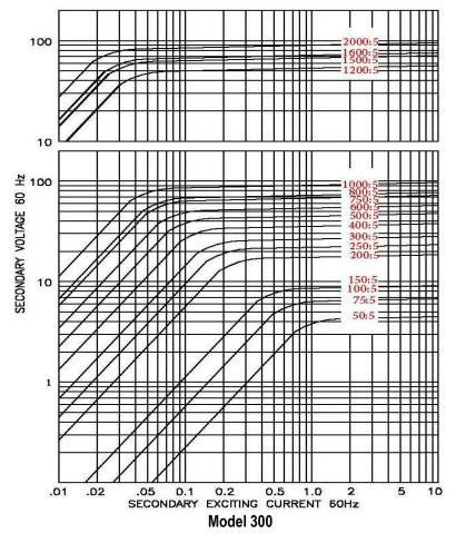
APPLICATION: Metering FREQUENCY: 50-400 Hz. NSULATION LEVEL: 600 Volts. 10 kV BIL. full wave WINDOW DIAMETER: 1.56" APPROXIMATE WEIGHT: 2.5 lbs.
