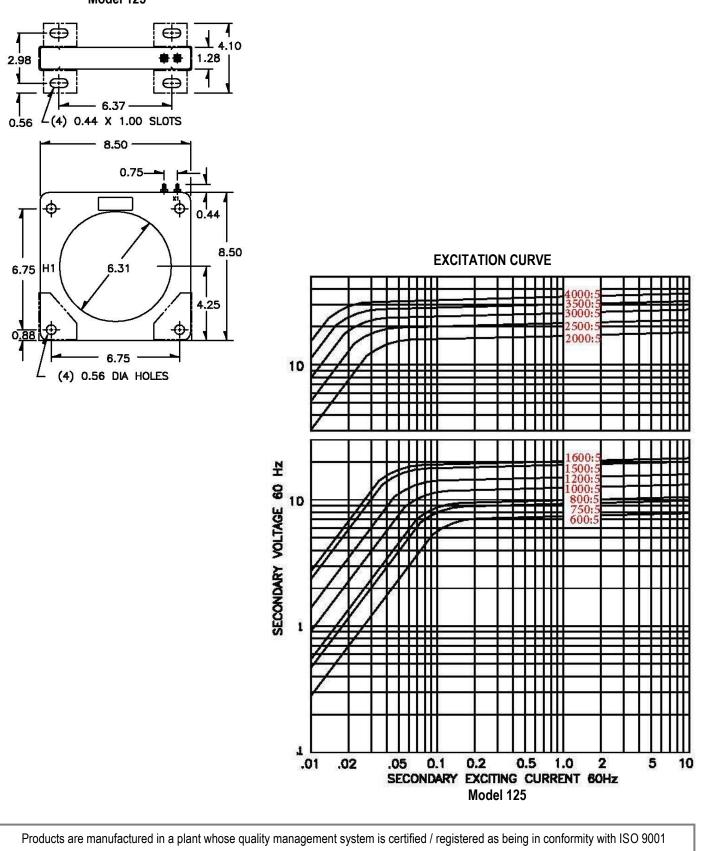
APPLICATION: Relaying and metering. FREQUENCY: 50-400 Hz. INSULATION LEVEL: 600 Volts. 10 kV BIL. full wave WINDOW DIAMETER: 8.13" APPROXIMATE WEIGHT: 22 lbs.
