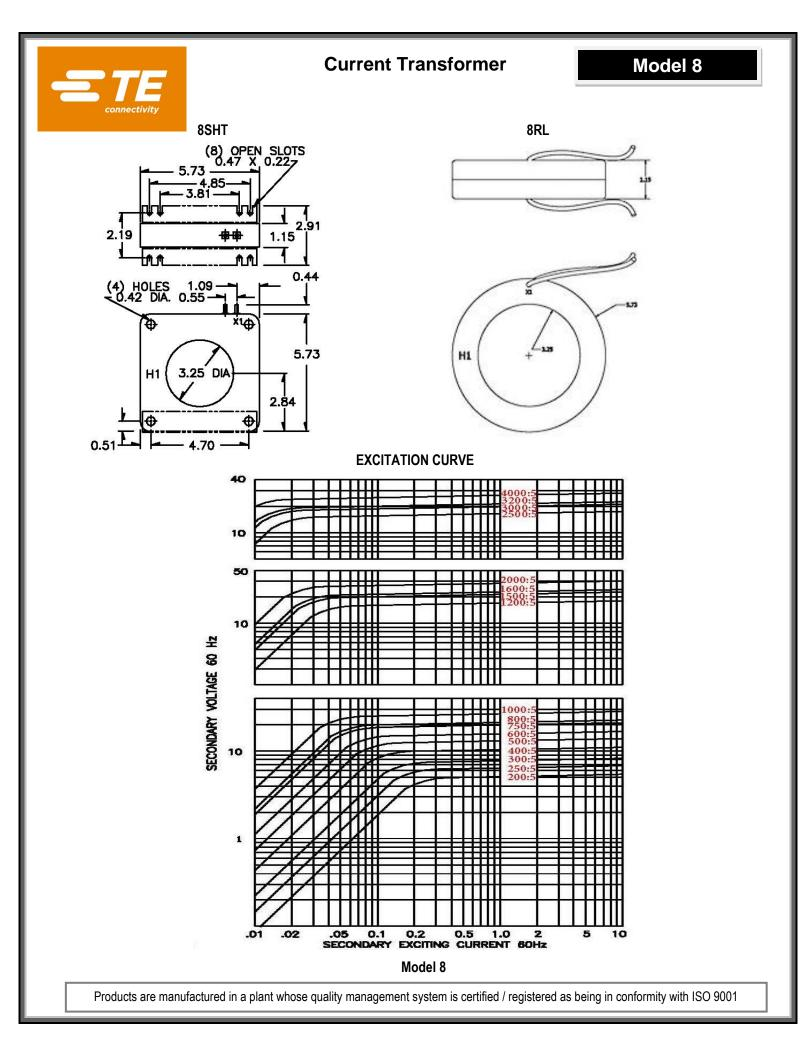
APPLICATION: Relaying and Metering FREQUENCY: 50-400 Hz. INSULATION LEVEL: 600 Volts. 10 kV BIL. full wave WINDOW DIAMETER: 4.0" APPROXIMATE WEIGHT: 9.5 lbs.
